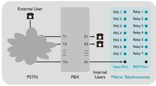
PBX extension connected to Input Port
